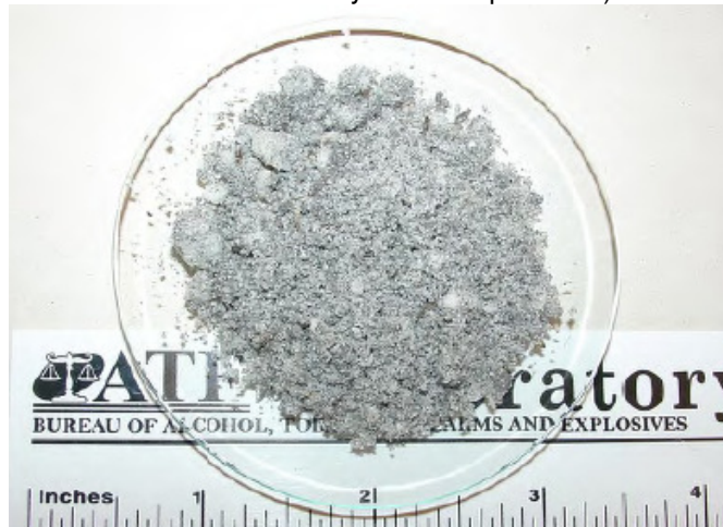
Sample of TATP mixture recovered from IED and sent to the ATF Lab to identify. Notice the high concentration of aluminum and the heterogeneous qualities of the mixture (1)
